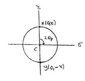
Determine the equivalent state of stress if an element is oriented 25° counterclockwise from the element shown.
