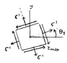
Determine the equivalent state of stress if an element is oriented 30° counterclockwise from the element shown.
