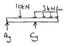
For the beam and loading shown, determine the maximum normal and maximum shear stresses at section n-n 2 m from the point A.
