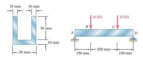
$$I = I_1 + I_2 + I_3 = 512.5 \times 10^{3} \text{ mm}^4$$
