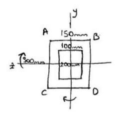
The box beam is subjected to the internal moment of  $M = 4 \text{ kN} \cdot \text{m}$ , which is directed as shown. Determine the maximum bending stress developed in the beam and the orientation of the neutral axis.
