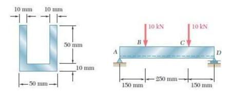
$$\mathcal{E}_{bottom} = -\frac{Mc}{I} = -\frac{(1.5 \times 10^3)(-0.025)}{512.5 \times 10^{-9}} = 73.2 \times 10^6 \text{ G}_{bottom}$$
