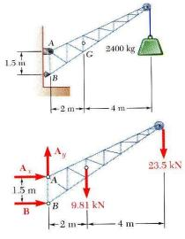
The first step in the static equilibrium analysis of a rigid body is identification of all forces acting on the body with a *free body diagram*.
