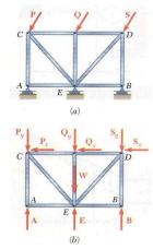
• Equal number unknowns and equations but improperly constrained
