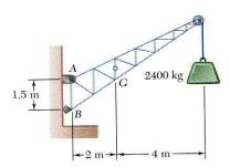
A fixed crane has a mass of 1000 kg and is used to lift a 2400 kg crate. It is held in place by a pin at *A* and a rocker at *B*. The center of gravity of the crane is located at *G*.
