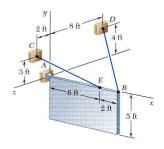
A sign of uniform density weighs 270 lb and is supported by a ball-and-socket joint at A and by two cables.
