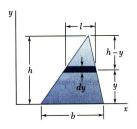
Determine the moment of inertia of a triangle with respect to its base.
