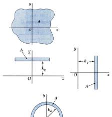
• Consider area A with moment of inertia  $I_x$ . Imagine that the area is concentrated in a thin strip parallel to the x axis with equivalent  $I_x$ .
