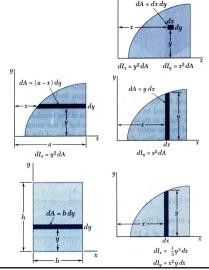
• Second moments or moments of inertia of an area with respect to the x and y axes,
