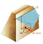
• Example: Consider the net hydrostatic force on a submerged circular gate.
