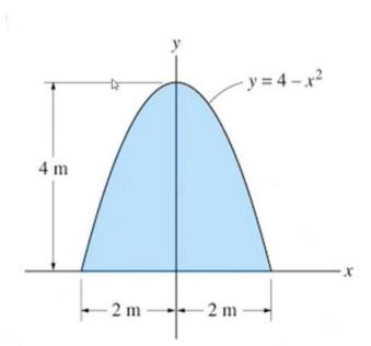
Calculate the moment of inertia of the shaded area about the x-axis.
