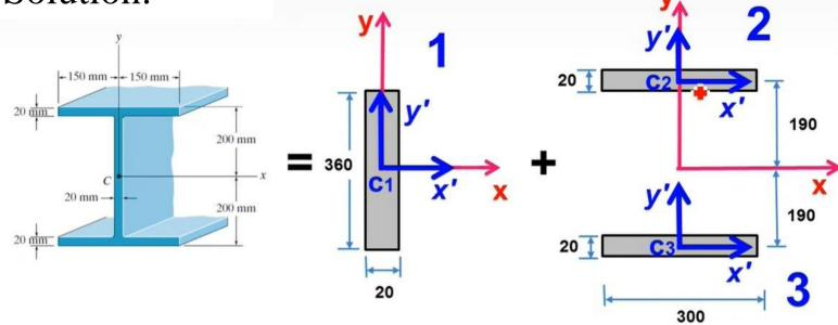
$$I_x = I_{x1} + I_{x2} + I_{x3} = I_{x1} + 2I_{x2}$$
