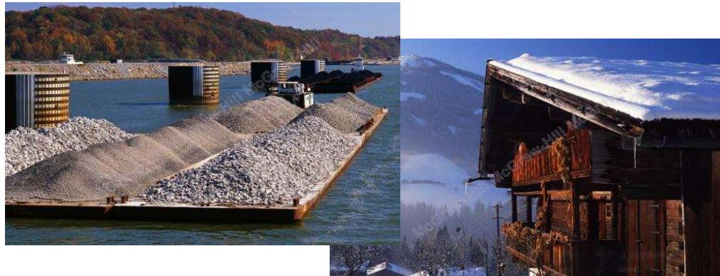
There are many examples in engineering analysis of distributed loads. It is convenient in some cases to represent such loads as a concentrated force located at the *centroid* of the distributed load.
