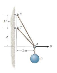
$$F_{AB} \xrightarrow{+} \Sigma F_{x} = 0; \quad 300 - F_{AB} \left(\frac{4}{\sqrt{41}}\right) - F_{AC} \left(\frac{2}{\sqrt{5}}\right) = 0$$
