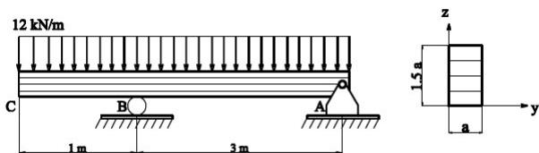
A laminated wooden beam of rectangular cross section supports a uniformly distributed load as shown. The beam is pin supported at A and simply supported at B. The beam cross section is to have a height-to-width ratio of 1.5. The allowable bending stress  $\sigma_{allow} = 9 \text{ MPa}$  and the allowable shear stress is  $\tau_{allow} = 0.6 \text{ MPa}$ . Neglecting the weight of the beam, calculate minimum allowable a value.
