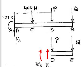
$$\begin{aligned} \sum F &= 0 \quad +\uparrow \\ V_A - 400 - P - Q &= 0 \quad M_A = -221.3 \text{ N.m} \\ V_A &= 1150 \text{ N} \end{aligned}$$
