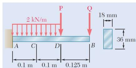
Beam AB supports a uniformly distributed load of 2 kN/m and two concentrated loads P and Q. It has been experimentally determined that the normal stress due to bending in the bottom edge of the beam is -56.9 MPa at A and -29.9 MPa at C.
