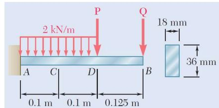
$$\begin{aligned}P &= 500 \text{ N}, Q = 250 \text{ N} \\M_C &= -116.3 \text{ N.m} \\M_A &= -221.3 \text{ N.m} \\M_D &= -31.25 \text{ Nm} \\V_A &= 1150 \text{ N} \quad V_D = 750 \text{ N}\end{aligned}$$
