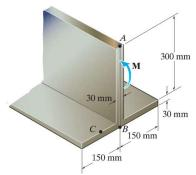
If the beam is subjected to an internal moment of M=100 kN.m, determine the bending stress developed at points A, B and C. Sketch the bending stress distribution on the cross section.)
