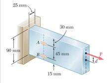
An eccentric force P is applied as shown to a steel bar of 25 90-mm cross section. The strains at A and B have been measured and found to be
