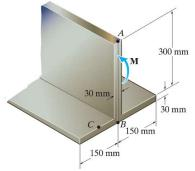
If the beam is subjected to an internal moment of M=100 kN.m, determine the bending stress developed at points A, B and C. Sketch the bending stress distribution on the cross section.)
