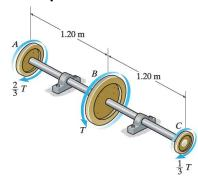
\*5–52. The 60-mm-diameter shaft is made of 6061-T6 aluminum. If the allowable shear stress is  $\tau_{\rm allow}=80$  MPa, and the angle of twist of disk A relative to disk C is limited so that it does not exceed 0.06 rad, determine the maximum allowable torque T.
