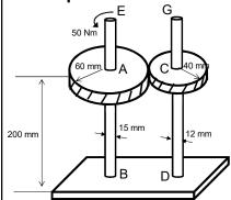
Rotation is prevented at B and D. A 50 Nm torque is applied at E of shaft
