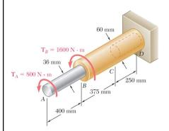
The aluminum rod AB (G = 27 GPa) is bonded to the brass rod BD (G = 39GPa). Knowing that portion CD of the brass rod is hollow and has an inner diameter of 40 mm, determine the angle of twist at A.
