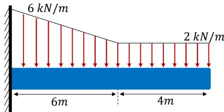
Determine the reactions at the beam supports for the given loadings.
