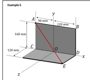
The wire AE is stretched between the corners A and E of a bent plate. Knowing that the tension in the wire is 435 [N], determine the moment about O of the force exerted by the wire (a) on corner A, (b) on corner E.
