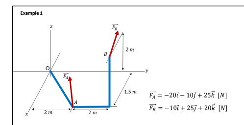
Replace the force system by a resultant force and a couple at point O.
