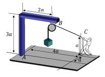
A rope passes over an ideal pully as shown in the figure. It carries a crate with weight W and held at point  $\mathcal{C}$ . The radius of the pulley may be neglected. Determine the resultant moment of the forces in the rope about point A.
