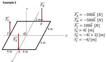
Replace the force system by a resultant force **only** and specify its points of application.
