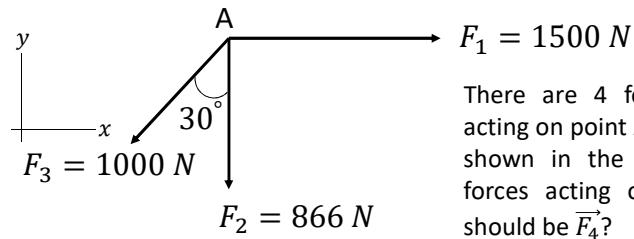
There are 4 forces ( $F_1, F_2, F_3, F_4$ ) acting on point A. 3 of the forces are shown in the figure. If the total forces acting on A is zero, what should be  $\vec{F}_4$ ?
