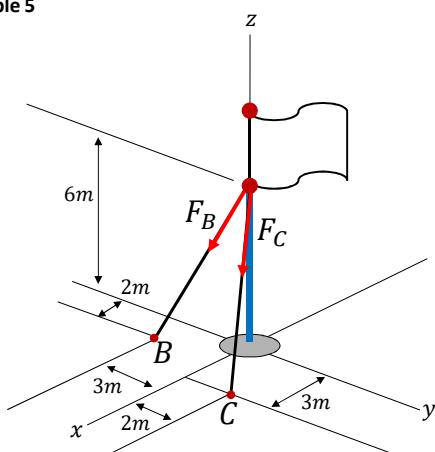
If  $F_B = 560 \text{ N}$  and  $F_C = 700 \text{ N}$ , determine the magnitude and coordinate angles of the resultant force acting on the flag pole.
