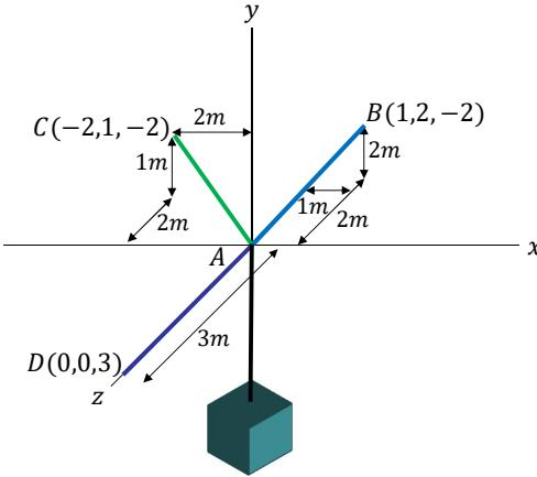
Determine the forces in cables AB, AC and AD required to support the 300 N crate.
