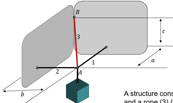
A structure consists of two bars (1 and 2) and a rope (3) (weights negligible). It is loaded in A by a box weight  $W$ . Determine the forces in the bars and the rope.
