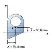
$$\overline{X} = \frac{\sum \overline{x}A}{\sum A} = \frac{+757.7 \times 10^3 \text{ mm}^3}{13.828 \times 10^3 \text{ mm}^2}$$
