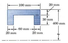
The outside diameter of a pulley is 0.8 m, and the cross section of its rim is as shown. Knowing that the pulley is made of steel and that the density of steel is  $\rho$ =7.85×10<sup>3</sup> kg/m<sup>3</sup> determine the mass and weight of the rim.
