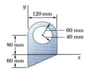
For the plane area shown, determine the first moments with respect to the *x* and *y* axes and the location of the centroid.
