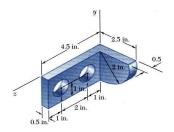
• Moment of the total weight concentrated at the center of gravity G is equal to the sum of the moments of the weights of the component parts.
