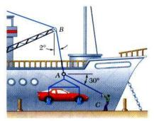
In a ship-unloading operation, a 3500N automobile is supported by a cable. A rope is tied to the cable and pulled to center the automobile over its intended position. What is the tension in the rope?
