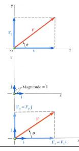
• It's possible to resolve a force vector into **perpendicular components** so that the resulting parallelogram is a rectangle.  $\vec{F}_x$  and  $\vec{F}_y$  are referred to as **rectangular vector components** and
