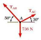
Free Body Diagram: A sketch showing only the forces on the selected particle. This must be created by you.
