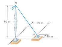
The tension in the wire is 2500 N. Determine:
