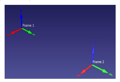
If you wish to modify the pose of any frame, double click on the frame from the tree or directly the frame in the scene to display frame details, from where you can edit the frame's name, its visibility, referencing, and pose. Another way of changing the pose of the frame is to press ALT, and it will change the display of the frame as
