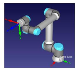
By default, it will be referenced to its own base reference frame; hence, if you move the base reference frame, whole body will move. In addition, a reference frame can be observed at the tip of the robot to easily control the movements of the tip. It is a preferred way for performing pick and place operations or similar.
