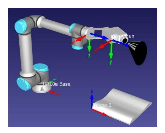
It is observed that the reference frame attached to the paint gun is positioned at the center of the gun. It is desired that this frame must be aligned with the surface of the spray. This can be achieved either through manually adjusting this frame's position and orientation while holding the ALT + SHIFT key, or directly from the Tool details dialog box. The reference frame most likely should resemble this
