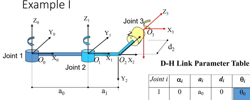
$\alpha_i$ : rotation angle from  $Z_{i-1}$  to  $Z_i$  about  $X_i$
