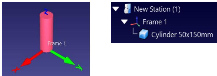
Now, by pressing the ALT key, it is possible to change the pose of the cylinder.
