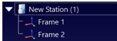
By default, Frame 1 is added at the center of the screen, the same origin as the station. Every subsequent frame added to the scene will be displaced by 1000mm along the Y-axis in reference to the station's reference frame which is considered parent to both Frame 1 and Frame 2.
